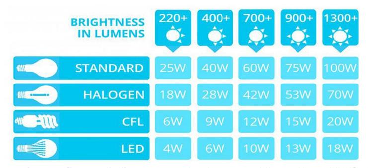
Traditional incandescent bulbs measure brightness in Watts. Since LED bulbs use far less energy than incandescent or CFL bulbs, their brightness is rated in Lumens. For example, a traditional 60-Watt light bulb emits over 800 Lumens. An LED equivalent may only measure 8.5 Watts, but it will still emit 800 Lumens and provide the same brightness levels.
